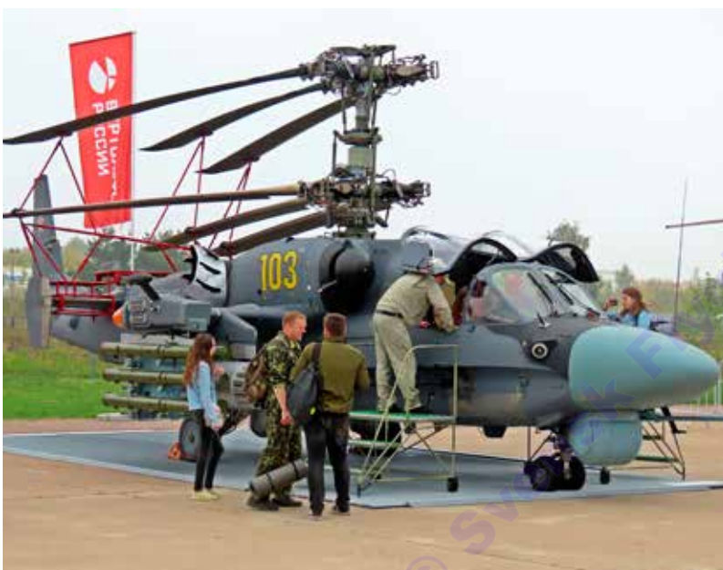
Attackhelikoptern Kamov Ka-52. Observera koaxialrotorn. Foto Lennart Samuelsson.
